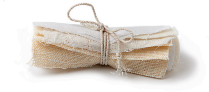
A single length of cloth torn in two. Scoured on the right, not scoured on the left.
